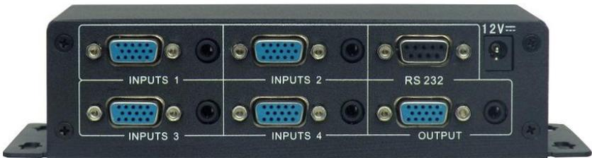
When the displaying input is removed under the auto-Sw mode, WVG4A will detect the 4 VGA inputs, ranging from input1, input2, input3, input4. When it finds a valid VGA signal, it will switch to this channel.
